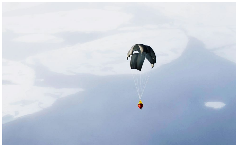
An Air-Deployable Expendable Ice Buoy deploys from a C-17 Globemaster III over the Arctic Ocean on July 12, 2023. The Office of Naval Research partnered with the 144 th Airlift Squadron to deploy data-gathering buoys across the Arctic Ocean. This deployment supported the International Arctic Buoy Programme, which maintains a network of buoys for real-time meteorological predictions and sea ice research. (U.S. Air Force photo by Airman 1 st Class Shelimar Rivera Rosado)
